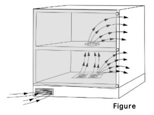
this possible is the ATM System 4, which includes a very powerful fan module. (Figure 2) Two stacks of three fans each produce a quiet but powerful air stream that can overcome substantial back pressure.
